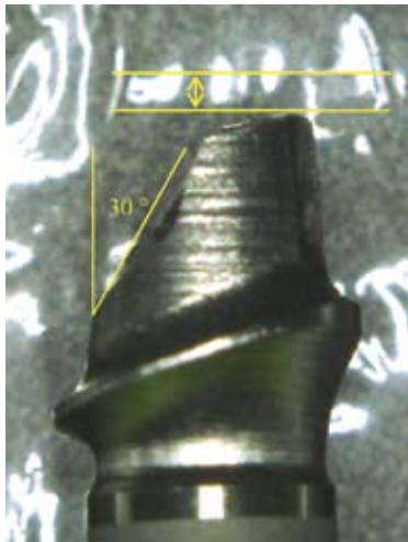
Fig 3. Prepared abutment section of the Zimmer One-Piece Implant showing reduced height (arrow) and increased angulation.
