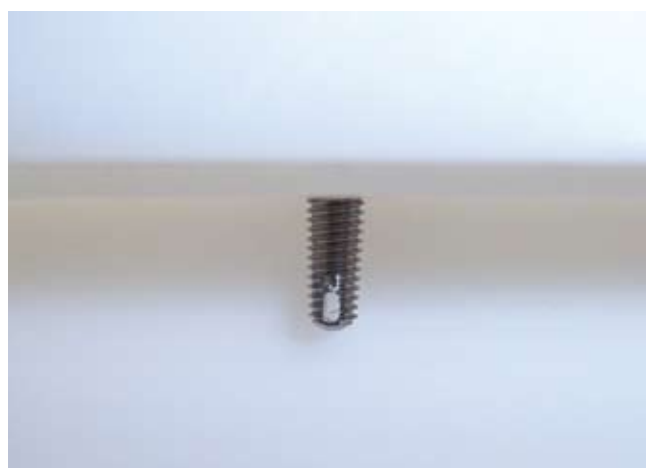
Fig 2. Threaded area of the implant is positioned for clear viewing by the infrared camera.
